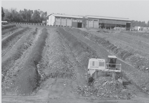
Figure B7.26.1 Turning the Windrows
